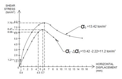
Figure 6. Shear stress computation based on the results of a direct shear test.
