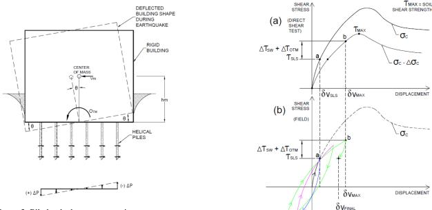
Figure 3. Pile loads due to overturning moment
